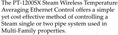
The PT-1200SX works by gathering temperature data from the Wireless Temperature Transmitters and performing an averaging calculation. The averaging result becomes the Building Average Temperature. The user configures a Day & Night temperature setpoint. When the Building Average Temperature drops below the setpoint. The system sends a "Call for Heat" to the Steam Boiler.
